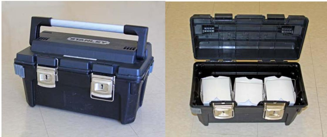
Figure 2. Larger covered plastic bin for secondary containment
